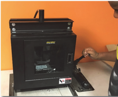
Left, an EZPC Recycling LLC employee demonstrates use of the SEM0101 utilized to destroy hard drives harvested from computers turned in as part of e-Waste. Below, EA’s 2018 e-Waste collection prior to transport to EZPC for destruction and recycling.
